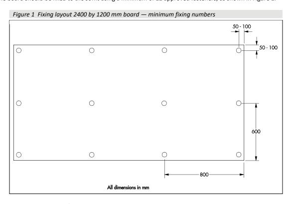
A.4 The distance between the fixings and the panel edge should not be less than 50 mm, or greater than 100 mm.
