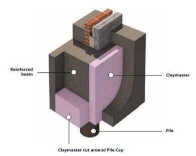
Claymaster boards are laid in the bottom of the trench, ensuring that the full width of the trench is lined and that the boards are butted tightly together.
