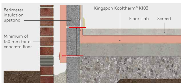
Figure 1: Complete masonry floor insulation
