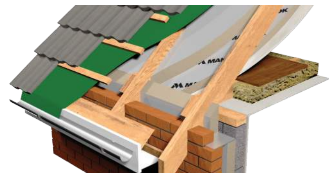
Pitched roof: MLK below rafters
