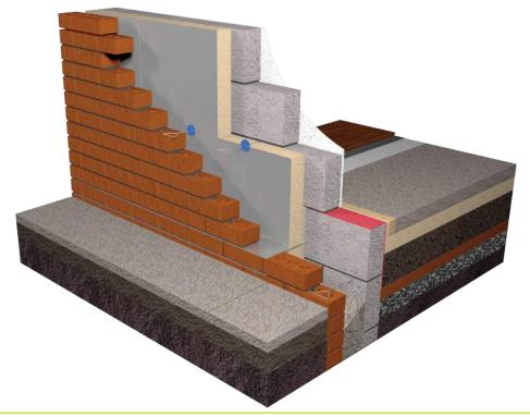
Cavity walls: MC in masonry - partial fill
