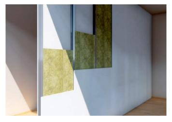
Studs: 70mm metal 'C 'studs at 600mm Centres Facings: 1 layer of 12.5mm standard plasterboard (total mass per unit area 8.0kg/m² each side)
