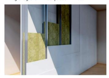
Studs: 70mm metal 'C 'studs at 600mm Centres 2 layers of 12.5mm standard plasterboard Facings:
