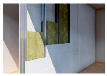
Studs: 70mm metal 'C 'studs at 600mm Centres Facings: 2 layers of 12.5mm standard plasterboard (total mass per unit area 20.0kg/m² each side)
