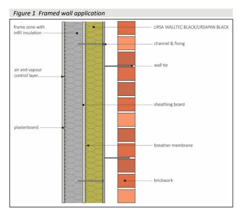
A.13 The insulation must be installed tightly against the sheathing board and secured to the frame studs, through the brick tie channels, using suitable screw or bolt fixings. The brick tie channels are installed at a maximum of 600 mm centres horizontally. The fixings must give a positive stand-off or incorporate a compression sleeve.
